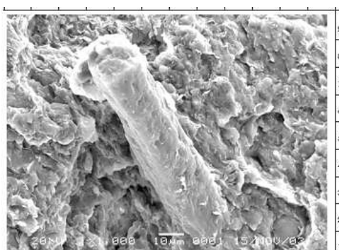
Figure 5.4.10. SEM photomicrograph of sporinite (D-H, 1-8) and oil droplet (K, 1-2), surrounded by kaolinite and smectite (montmorillonite). X1000. Sample 03NS13A.
