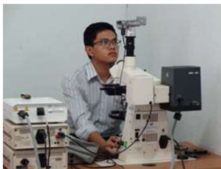
Figure 3.2. A Leitz MPV-2 photomicroscope in Tekmira Laboratory used to analyze maceral observation, including type of macerals, vitrinite reflectance, and thermal alteration index, all in reflected white light and on fluorescence modes.
