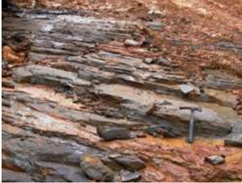
Figure 4.4.6. Outcrop of semi-fresh shale and mudstone intercalations, within road-cut cliff, nearby PT. Nusa Riau coalfield. The upper part of shale layer shows thick-bedded, flaggy character, grey, containing thin intercalations of Fe-oxides, presumably occur as weathered tuffaceous material.
