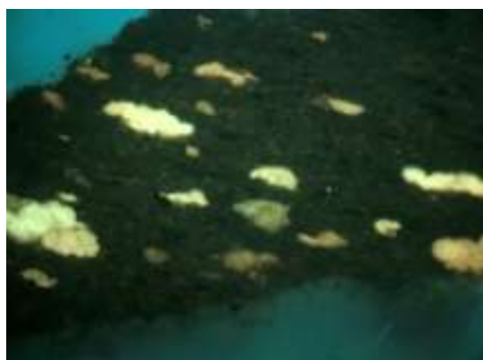
Figure 5.10.1. Photomicrograph of telalginite- Botryococcus embedded within Sinamar sediments. Sample 08MH13. Fluorescence mode.
