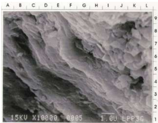
Figure 5.6.8. SEM photomicrograph of shale showing typical lamalginite (A-E, 1-2) and kaolinite (E-I, 3-9). Sample 00NS08G. Location: Karbindo Coalfield
