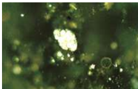
Figure 4.1.12. Photomicrographs of framboidal pyrite embedded within clay mineral matrix of the Butar Formation. X200. Reflected light. Sample 02HR14C. Reflected light. Location: Laubuluh.
