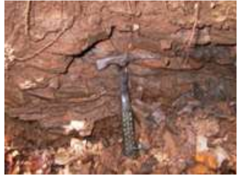
Figure 4.3.1. Outcrop of well bedded shale, brownish grey, flaky to flaggy, rather soft, oxidated, slightly weathered, outcropping in Jao River.
