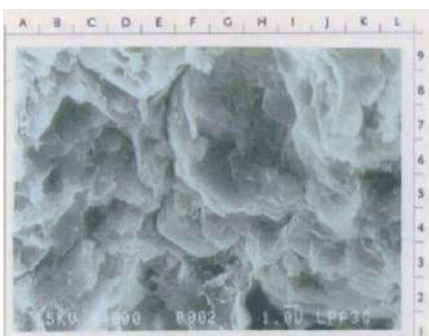
Figure 4.5.12. SEM photomicrograph showing kaolinite (F-L, 5-9 and E-G, 3-4) surrounded by smectite-illite (A-L, 1-9), calcite (H-I, 7-8) in oil shale of the Sangkarewang Formation. Sample 01NS08 1 . Location: Sipang River.
