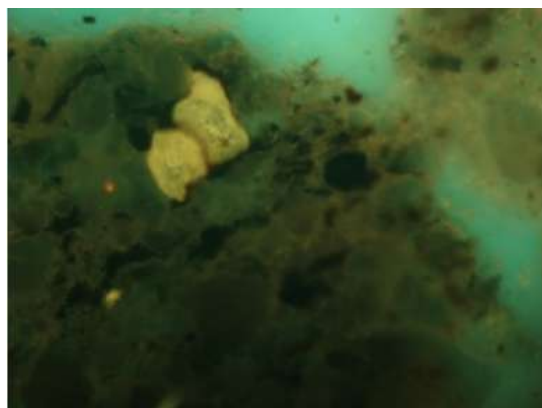
Figure 5.10.4. Photomicrograph of (?) bitumen contained within Sinamar sediments. Sample 08MH13E. Fluorescence mode.
