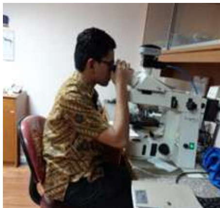
Figure 3.1. A Leitz MPV-2 photomicroscope in GRDC (Geological Research and Development Centre; now Centre of Geological Survey) Laboratory used to analyze maceral observation, including type of macerals, vitrinite reflectance, and thermal alteration index, all operated in reflected white light and on fluorescence modes.
