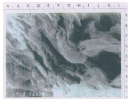
Figure 4.5.13. SEM photomicrograph of “smectite-illite” (A-E, 1-9 and F-L, 13) with alga of typically Pediastrum -lamalginite (F-L, 4-4) in oil shale of the Sangkarewang Formation. Sample 01NS08A. Location: Sipang River.
