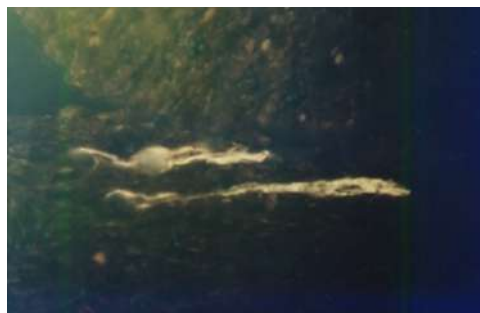
Figure 4.4.8. Photomicrograph of lamalginite (Al). (Fluorescence mode). X350. Sample 03NS16C.
