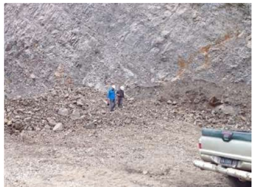
Figure 4.6.6. Highly dipping northwards, well-bedded thick shale-mudstone of Kiliran Formation, in the PT. Karbindo Apsyapradhi Coal Mines.
