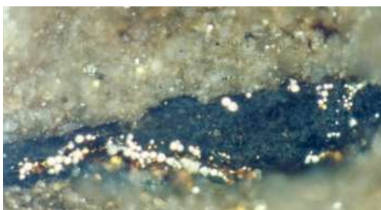
Figure 5.6.10. Photomicrograph of vitrinite (V) contains framboidal pyrite (Py), embedded in silty claystone (Cl) of the Kiliran Formation. (Reflected white light). Sample 00NS08N2. Location: Karbindo Coal Mines, Kiliranjao.
