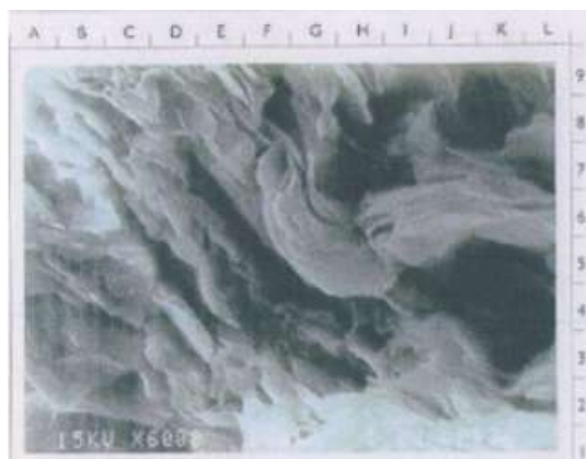
Figure 5.5.4. SEM photomicrograph of "smectite-illite" (A-E, 1-9 and F-L, 13) with alga of typically Pediatrum -lamalginite (F-L, 4-4) in oil shale of the Sangkarewang Formation. Sample 01NS08A. Location: Sipang River.
