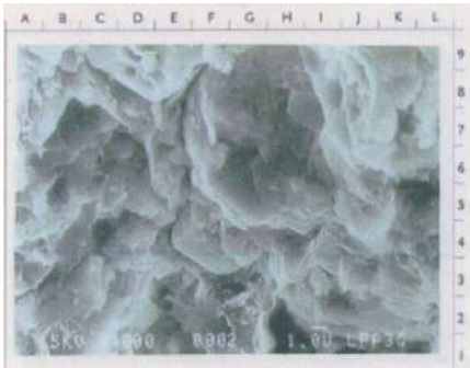
Figure 4.5.11. SEM photomicrograph showing kaolinite (F-L, 5-9 and E-G, 3-4) surrounded by smectite-illite (A-L, 1-9), calcite (H-I, 7-8) in oil shale of the Sangkarewang Formation. Sample 01NS08 1 . Location: Sipang River.
