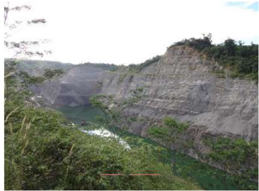
Figure 4.6.4. Thick cut-off sequence of shale and interbedded mudstone of Kiliran Formation, outcropping in the PT. Karbindo Apsyapradhi Coal Mines.
