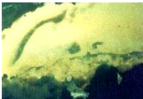
Figure 5.3.1. Photomicrograph of bitumen in the Keruh oil shale derived from algae. Size of bitumen around 20 micron. Location: Diano River.
