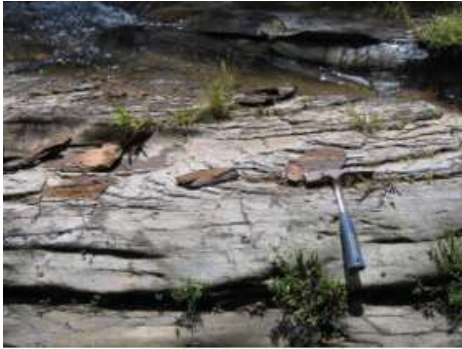
Figure 4.11.10. Photograph of outcrop of Kasiro mudstone unit, showing thin to thick bedded-flaggy structure; hard, compact. Location: Sekeladi River. (Suwarna, 2005).
