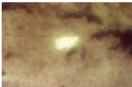
Figure 5.6.13. Photomicrograph of telalginite- Botryococcus embedded within clay matrix.
