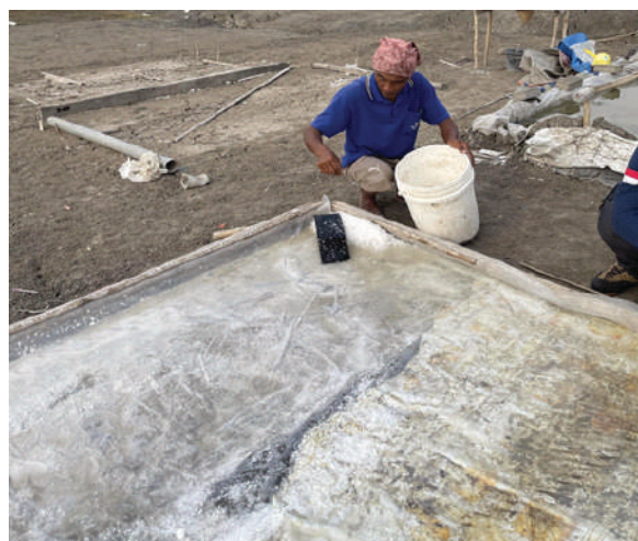
Figure 12.4 The traditional processing of brine water through evaporation to obtain lithium-rich salt at Bledug Kuwu (CMCGR, 2023)
