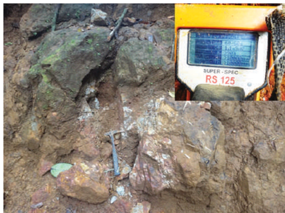
Figure 11.1 Outcrop: U-Th-REE Mineralization in Britholite Formation at Mamuju Area, exhibiting a dose rate of 1.1 mSv/h (Sukadana et al., 2022)
