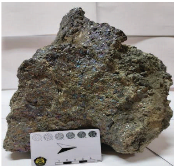
Figure 3.2 Copper mineralization; chalcopyrite, bornite, and azurite vein-type (epithermal) in the Dunu area, Monano District, North Gorontalo Regency, Gorontalo Province (Nugraha, et al., 2023)
