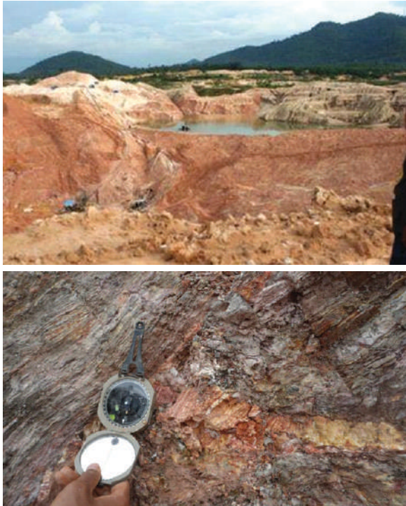
Figure 6.1 Alluvial Tin Mining Landscape in Indonesia: Evidence of Secondary Tin Deposition (Top), Structural Mapping of Hydrothermal Veins in Primary Tin Deposit (Bottom) (GAI, 2021)
