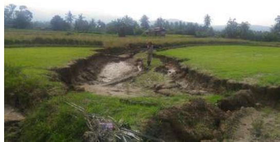
Figure 1.3. Lateral spreading observed in the Jono Oge area.
