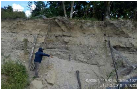
Figure 4.3.20. The outcrop of the Petobo landslide crown showing alternating layers of gravel - pebbles (sediment gravity flow products) and sand (sand bedforms products) (Source: Buana, 2018).
