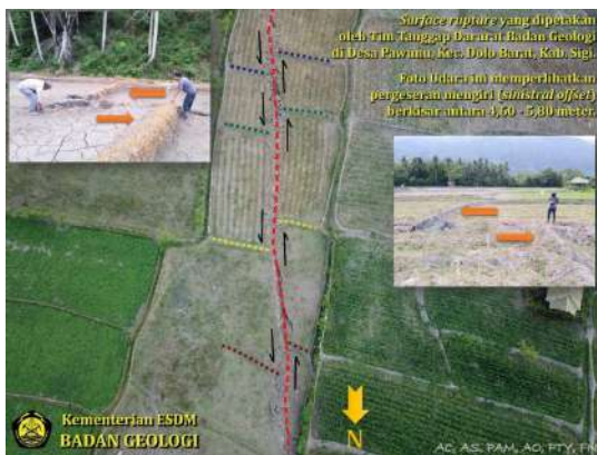
Figure 3.11. Sinistral offset of fault surface rupture around 4,6 m to 5,8 m caused by earthquake on September 28 th , 2018 in Pawunu Village, Dolo Barat District, Sigi Regency (Supartoyo et al. , 2018).
