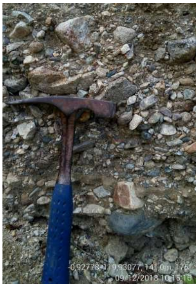
Figure 4.3.22. Gcm facies outcrop in the upstream part of the Petobo affected area which is analogous to the lithology of the KPE alluvial fan (Source: Buana, 2018).
